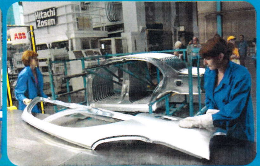
ASSEMBLING THE CAR BODY AT THE «COSKUNOZ ALABUGA»
